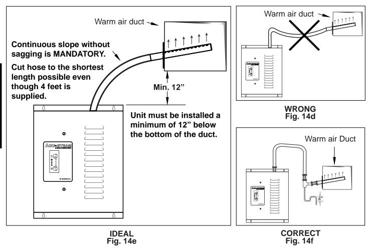
**NOTE**: If it is not possible to get enough slope for the condensation to return properly to the water tank, then an S-shaped steam trap (not supplied) must be installed at the lowest point of the steam hose. This steam trap hose should have a minimum height of 4". Please see <u>Fig. 14f</u>.
