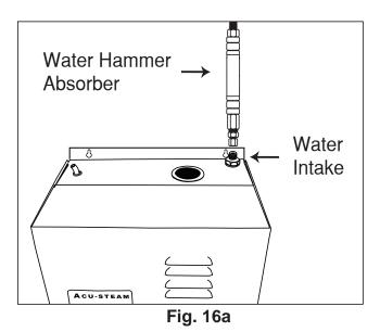
16.2 At the other end of the water hammer absorber, connect the water supply tube, using the same type of fitting used on the water supply valve. Tighten the compression nut, without stripping, with two wrenches, one to hold the water hammer end, and one to turn the compression nut. Please see <u>Fig. 16b</u>.
