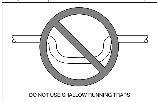
Figure 15 Insufficient Condensate Trap
