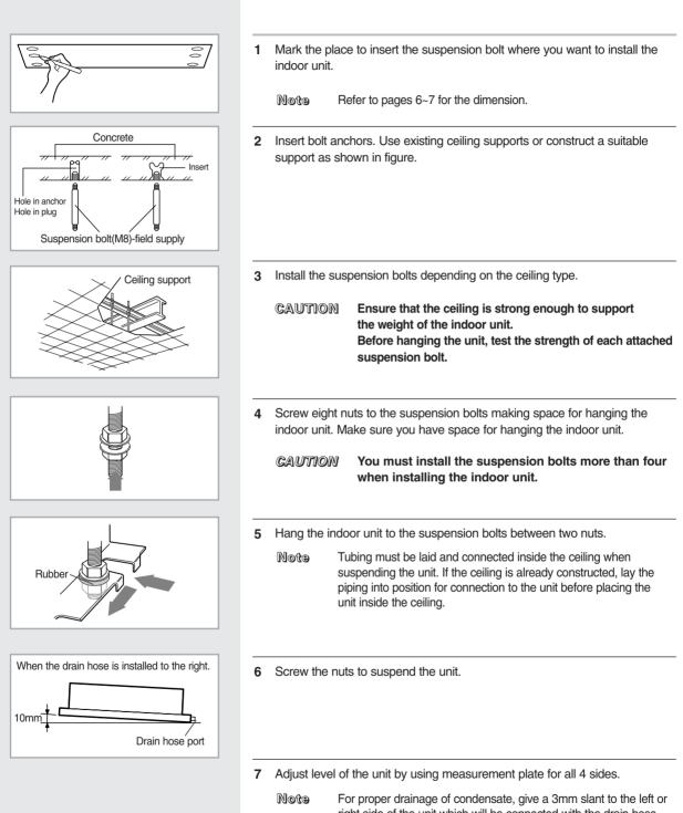
For proper drainage of condensate, give a 3mm slant to the left or right side of the unit which will be connected with the drain hose, as shown in the figure. Make a tilt when you wish to install the drain pump, too.
