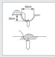
If the power distribution circuit does not have an earth or the ground does not comply with specifications, an grounding electrode must be installed. The corresponding accessories are not supplied with the air conditioner.
