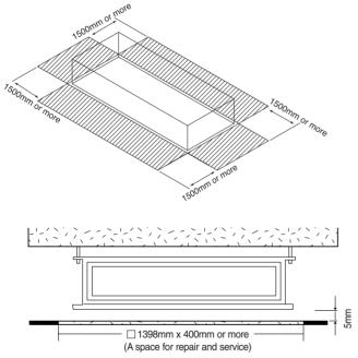
You must have 5mm or more space between the ceiling and the bottom of indoor unit. Otherwise, the noise from the vibration of indoor unit may bother the user. When the ceiling is under construction, the hole for check-up must be made to take service, clean and repair the unit.
