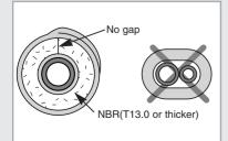
Once you have checked that there are no leaks in the system, you can insulate the piping and hose.
