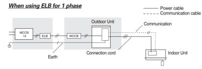
\* If an outdoor unit is installed in a place in danger of an electric leak or submergence, you must install the ELB.
