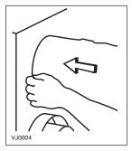
Pull the vapor barrier over the insulation and over the outer ring of the double collar.
