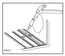
From the inside of the unit, punch both knock-out sections located at the bottom of the unit.
