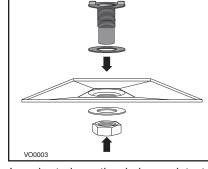
In order to keep the drain pan intact, hand tighten both plastic drain fittings to the unit using the gaskets, washers and nuts as shown.
