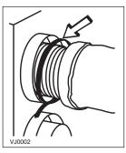
Attach the flexible duct to the port using tie wrap.
