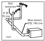
End branches: Each end branch will have to transport a 70 cfm air flow (140 divided by 2). Table on page 5 indicates for a 5" Ø duct: recommended air flow: 75 cfm; maximum air flow: 110 cfm. The high speed air flow of 70 cfm is close enough to the recommended value (75) and far away enough from the maximum value (110). Therefore, a 5" Ø duct or larger is an appropriate choice for both end branches.
