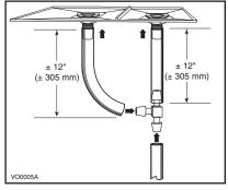
Cut 2 sections of the plastic tube, about 12" (305 mm) long, and attach them to each drain fitting. Join both short sections to the "T" junction and main tube as shown.
