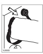
Apply duct tape to the joint making an airtight seal. Avoid compressing the insulation when pulling the tape tightly around the joint. Compressed insulation loses its R value and causes water dripping due to condensation on the exterior surface of the duct.
