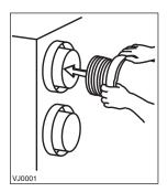
Pull back the insulation to expose the flexible duct.
