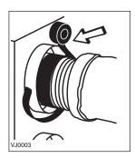
Pull the insulation over the joint and tuck in between the inner and outer rings of the double collar.
