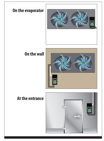
for easy viewing of the room temperature and/or system status. See **Figure 1** for locations.
