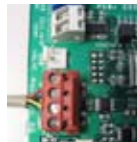
Figure 3. AquaLink RS 485 Communication (4-Wire Connection)
